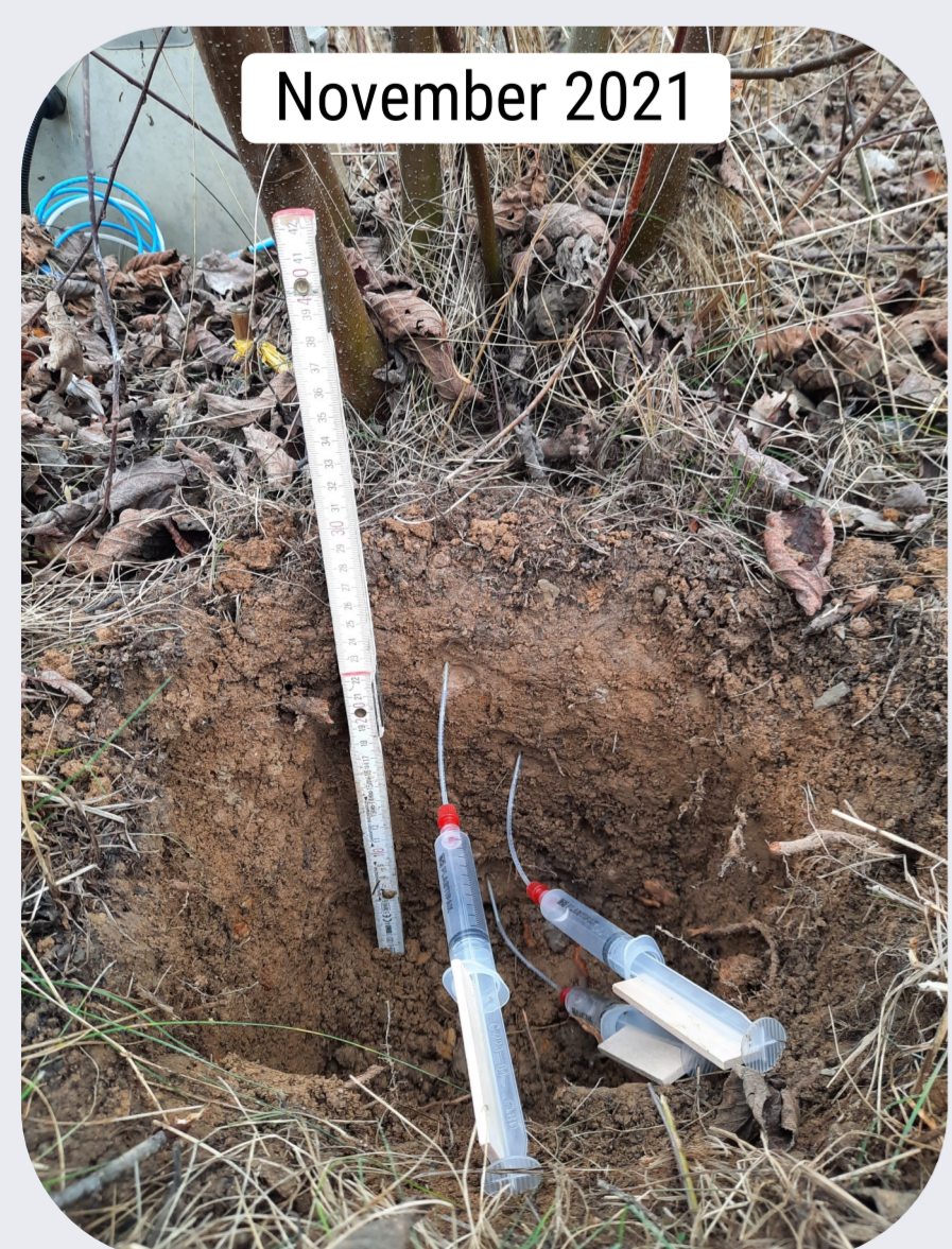
Sample collection of porewater with mini suction cups directly in the rhizosphere
